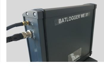
4. Switch the BATLOGGER on and check the LED
