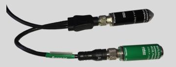
2. Connect the LTE and microphone/sensor cable
