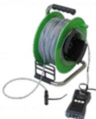
In order to record at greater distance to the BATLOGGER the extension kit green 100m can be used instead of the supplied microphone. The special microphone FG green can be located up to 100 meters away. For example, it is possible to attach the microphone on the top of a measuring mast, while the BATLOGGER can be placed protected and easily accessible on the ground.
